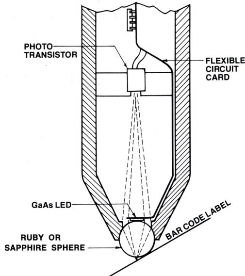
Schematic of Intermec's RUBY WAND Scanner
